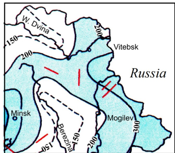
Figure 7 - Part of the depth map of the freshwater base in the north-eastern part of Belarus, Kudelsky et al. (2000). The red lines indicate local faults. Curves of isolines show the limits of groundwater occurrence within the region.
